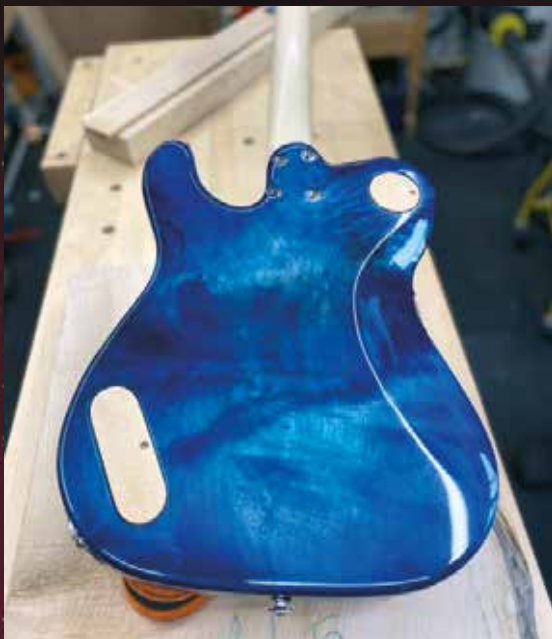
Back body, the finished shaping
